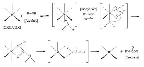
As shown in above figure, urethane formation occurs as a hydroxyl group, and then an isocyanate group is coordinate bonded to ORGATIX. In general, however, coordinate bonding between ORGATIX and a hydroxyl group is initiated promptly; hence it is common practice in urethane formation to add polyol, isocyanate and a catalyst at the same time.
